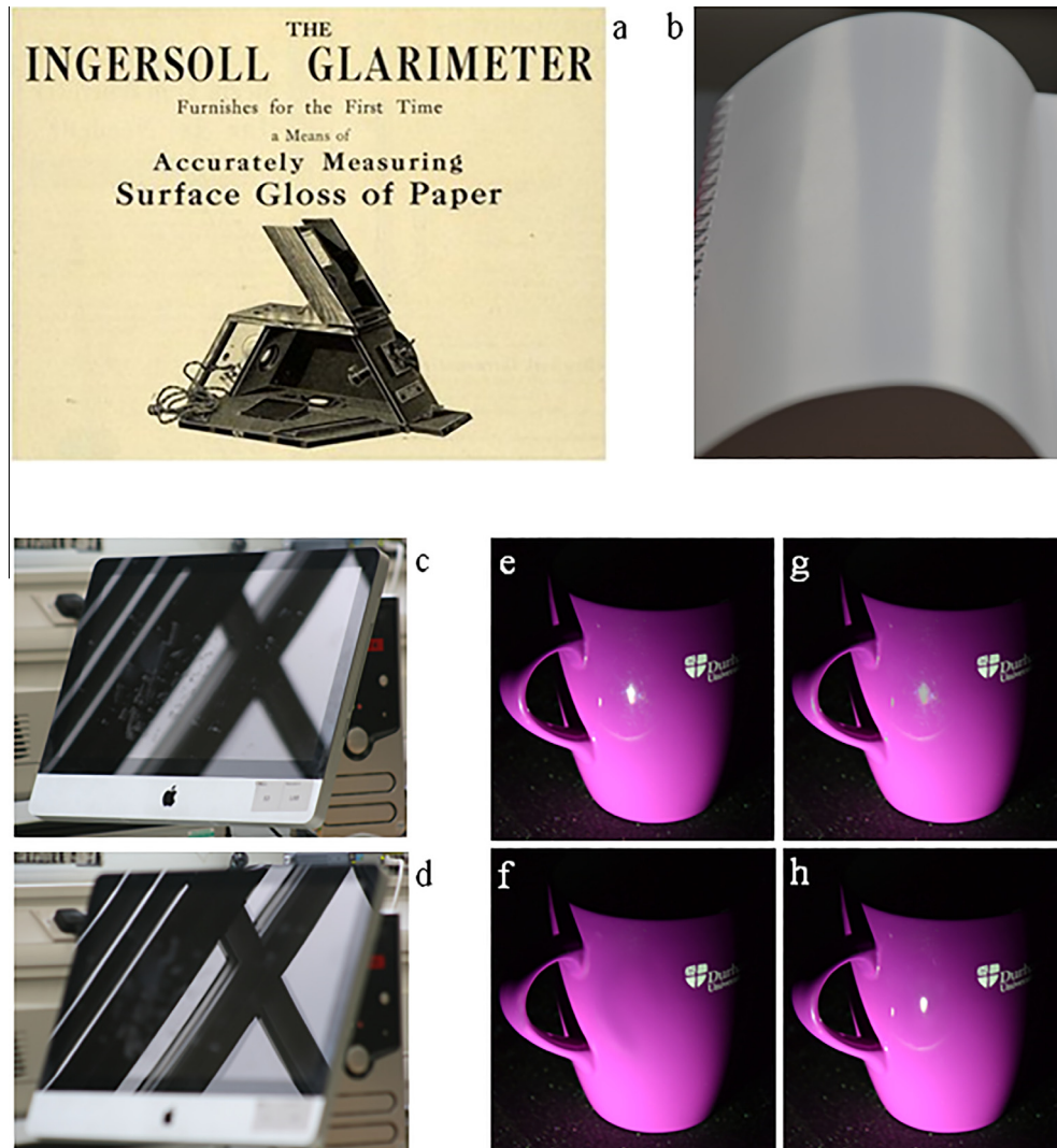
Fig. 1. (a) An advertisement for an Ingersoll Glarimeter, 1922. Reproduced under the Creative Commons license. (b–h) Illustrate examples of Hunter's six cues to gloss. (b) Shows sheen at grazing angles, on a piece of high quality matte paper. (c and d) Demonstrate both surface texture and distinctness-of-image gloss: (c) is focused on the fingerprint-blemished surface, whereas (d) is focused on the reflected image – the surface appears less glossy in (c) as the surface texture of the blemishes detracts from the surface gloss, and the distinctness of the reflected image is lower. (e) Shows the original photograph of a shiny surface with a strong highlight. In (f) all highlights have been removed, and the surface looks matte. In (g) the highlight has been reduced to demonstrate contrast shine, and in (h) all haze surrounding the highlight has been removed from the original image.
